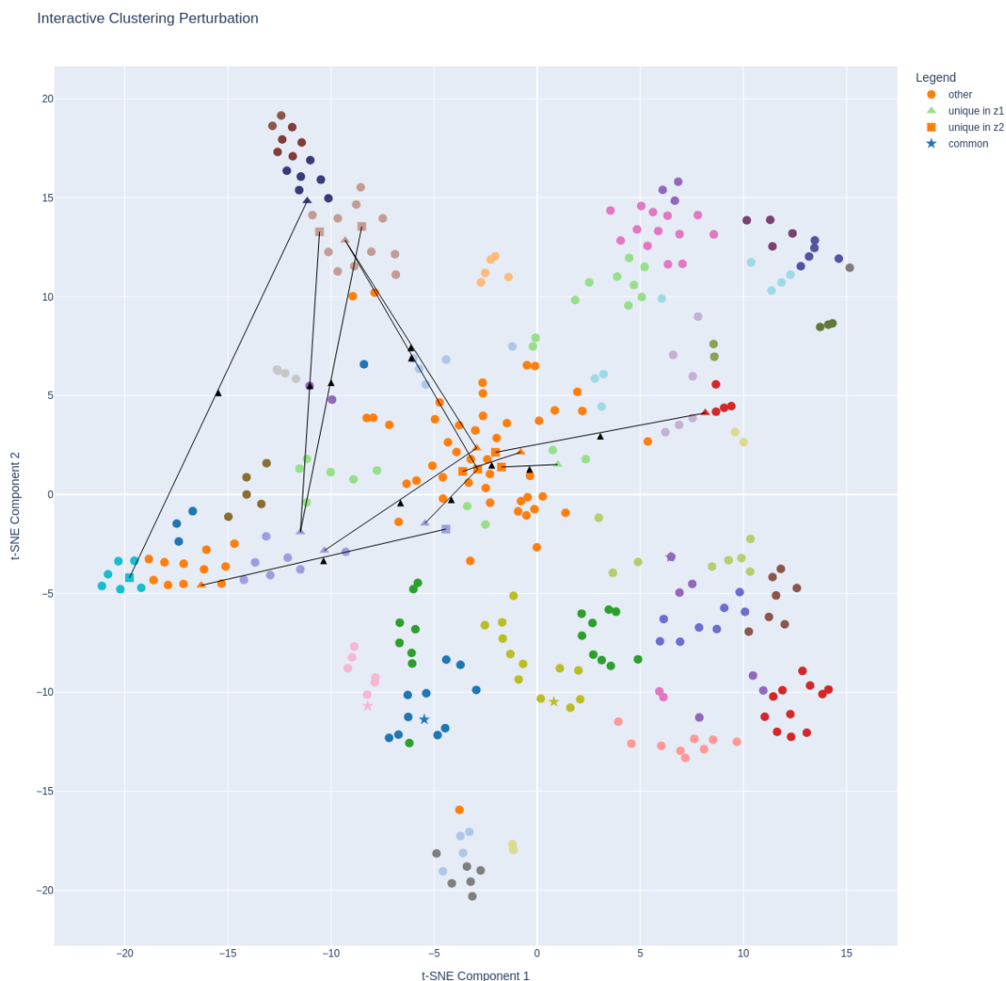
Figure 4.5: Visualization of clustered codebook vectors projected to 2D using t-SNE. Colors indicate cluster membership, while shapes denote categories. Lines connect vectors \mathbf{z}_1^i and \mathbf{z}_2^i for positions i where \mathbf{z}_1^i \neq \mathbf{z}_2^i . Hovering mouse over individual elements displays additional details, such as cluster membership, codebook index, and position in the discrete representation. The corresponding “directed” perturbation with reconstructed images is shown in Figure 4.4.
